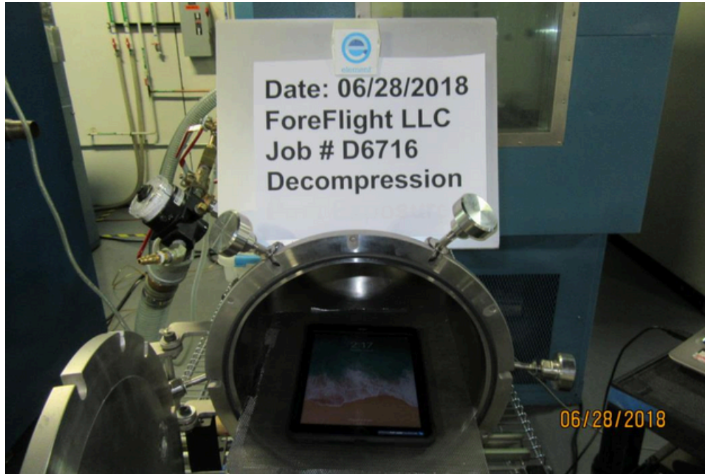
Photo 1 – Example of setup within pressure vessel, functional
